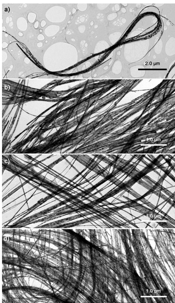
Figure 1. a–c) TEM images of CdSe nanowires doped with 2.1 %, 2.6 %, and 3.0 % Mn. d) TEM image of Mn-doped CdSe nanowires prepared by using double the amounts of Cd and Se precursors.
